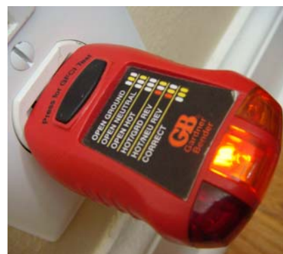
LHA inspectors use GFCI testers to ensure outlets are properly installed.
